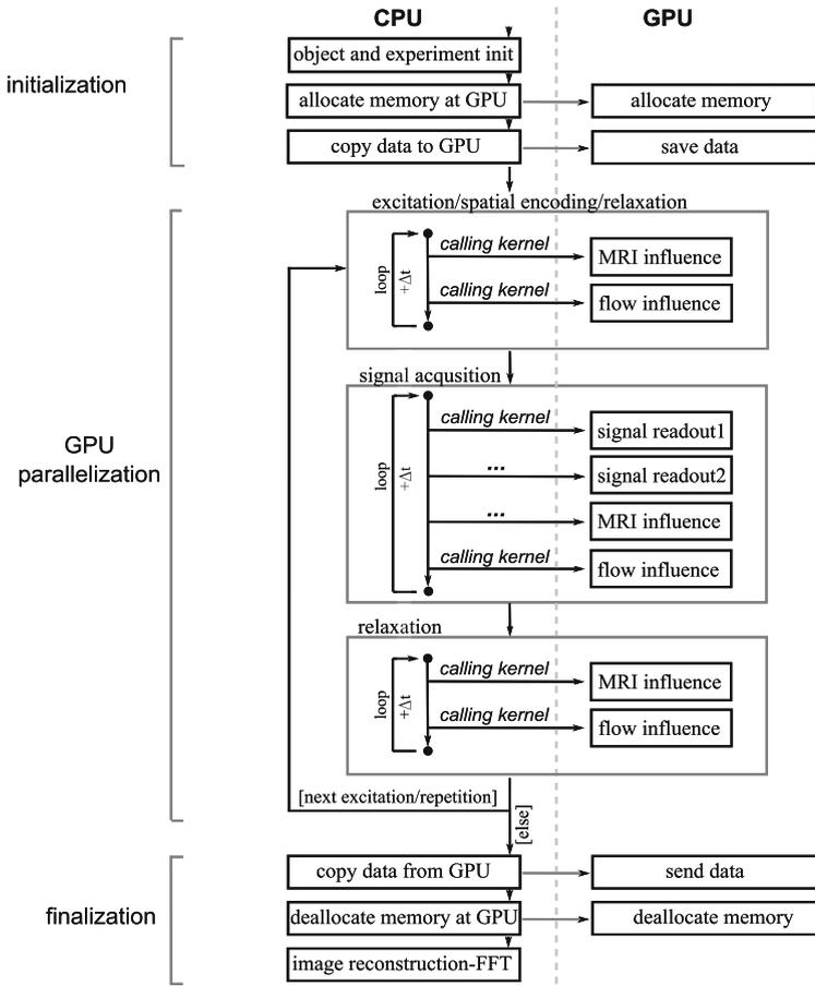
**Fig. 4.** The flowchart of the GPU-based algorithm of MR flow imaging
