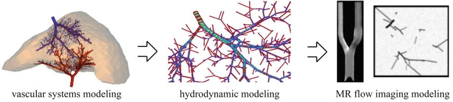
**Fig. 1.** Three-component MRI model overview. The model allows us to generate vascular structures, then simulate flow behaviour and finally reproduce MRI processes.
