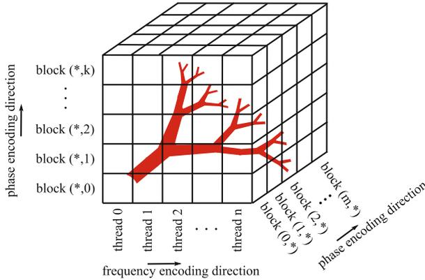
**Fig. 3.** Data decomposition strategy: 2D grid of blocks along the phase encoding directions and 1D block of threads along the frequency encoding direction.
