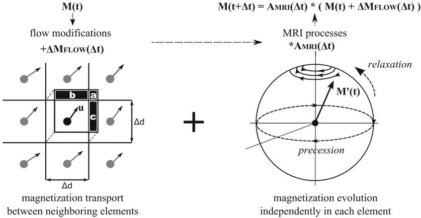
Fig. 2. The connection of MRI and magnetization transport algorithms.
