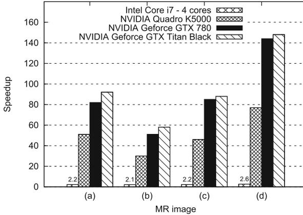
**Fig. 6.** Speedup of the GPU (as well as multi-core) accelerated algorithms relative to the serial implementation run on a single core of Intel Core I7 CPU. Images shown in Fig. 5 and various GPUs are tested.
