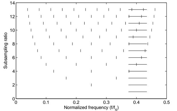
Fig. 6 Relation between 16-th subband and integer band positions corresponding to subsampling
