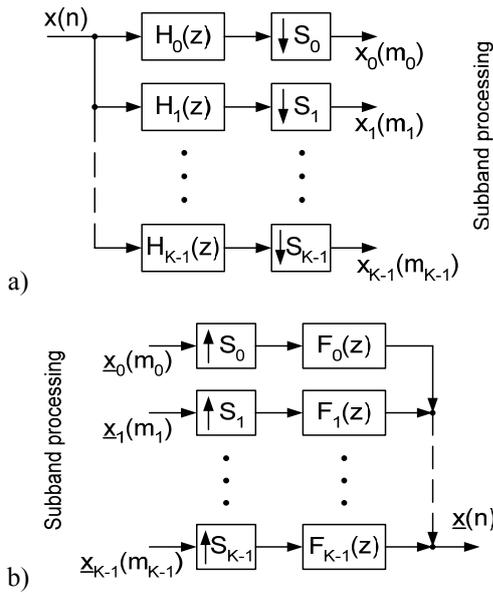
Fig. 2 General schema of analysis (a) and synthesis (b) multirate filter bank
