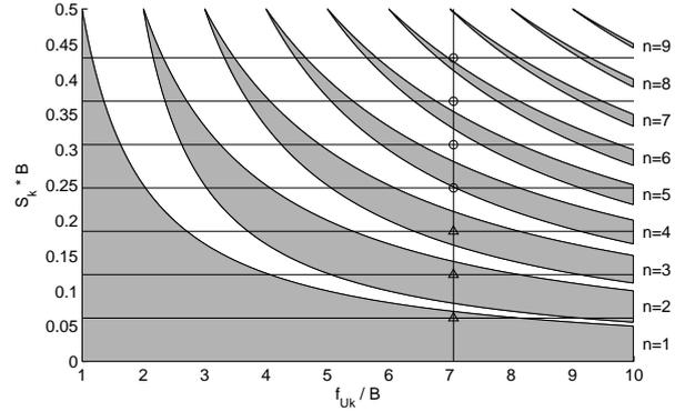
Fig. 5 Allowed subsampling ratios vs. subband position
