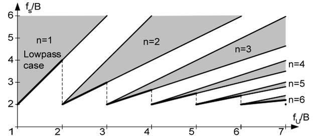
Fig. 1 Allowed sampling rates vs. band position
