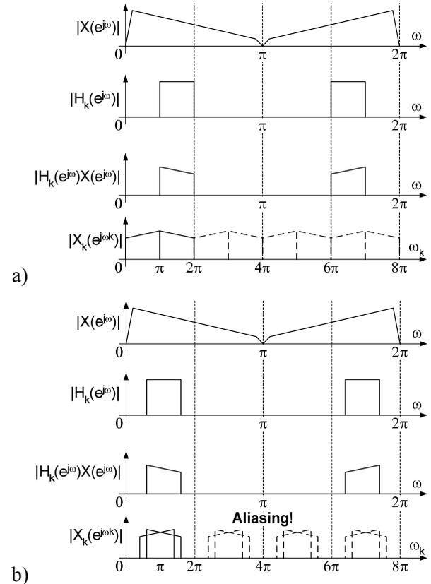
Fig. 4 Subsampling of integer (a) and arbitrary (b) positioned subband in cosine modulated filter bank
